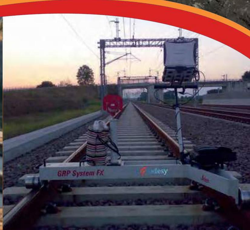
Rail Tracks Set-Up - Construction Surveying - Laser Scanner
